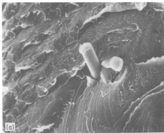
Figure 9 Electron scanning micrographs of the fracture surfaces of: (a) ULTEM-fibres, (b) PES-fibres composites; (c) carbon fibres after extraction with toluene. \times 750 .
